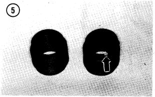
8. If heat was necessary to remove shift lever screw, check washer located under lever for damage. Replace as required.
